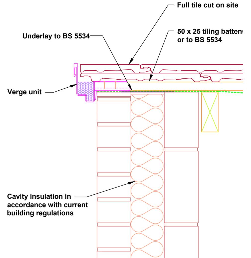
**Note: When using a vapour permeable (LR) underlay, Forticrete in line with BS5250 recommend that the batten cavity is ventilated from eave to ridge**
